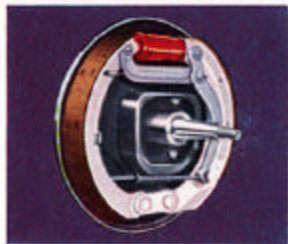
Pistons in double hydraulic cylinder move two independently-anchored brake shoes into smooth, firm contact with each brake drum.
